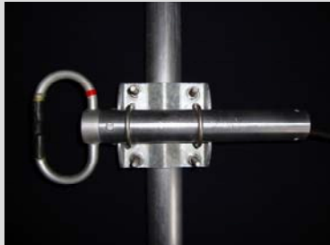
1/4 - wave spacing (6.95 – 7.5 dBd gain) (Offset pattern)
